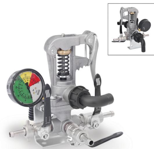
**Remote control unit** with working pressure regulating valve, bar feeding opening/closure control lever, anti drip and glycerine bath pressure gauge with coloured dial, with differential scale isometric pressure gauge on request. Self-cleaning delivery line filter supplied on request.
